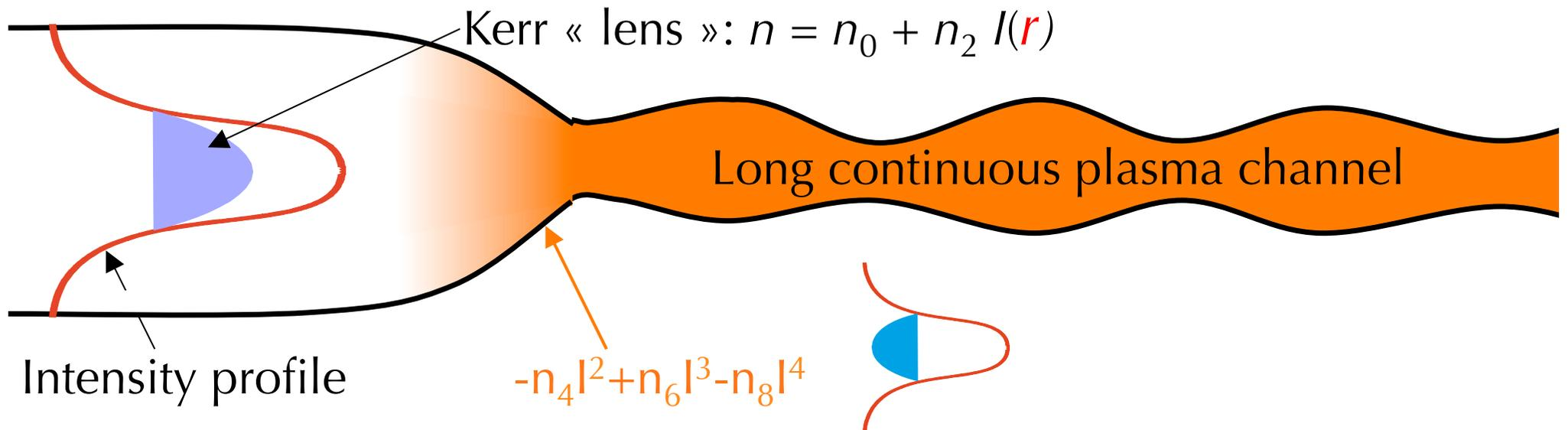
Filament:  $\Phi = 100 \mu\text{m}$ ,  $L > 100 \text{ m}$ ,  $I = 10^{14} \text{ W/cm}^2$ ,  $\rho = 10^{15} \text{ cm}^{-3}$
