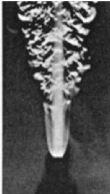
Schlieren photo of a turbulent flame of an oxy-acetylene torch<sup>1</sup>
