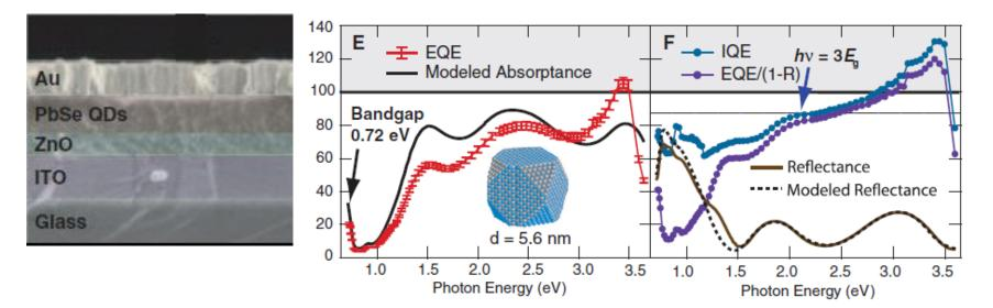
**EQE, External Quantum Efficiency:** Quantum efficiency of the whole device
