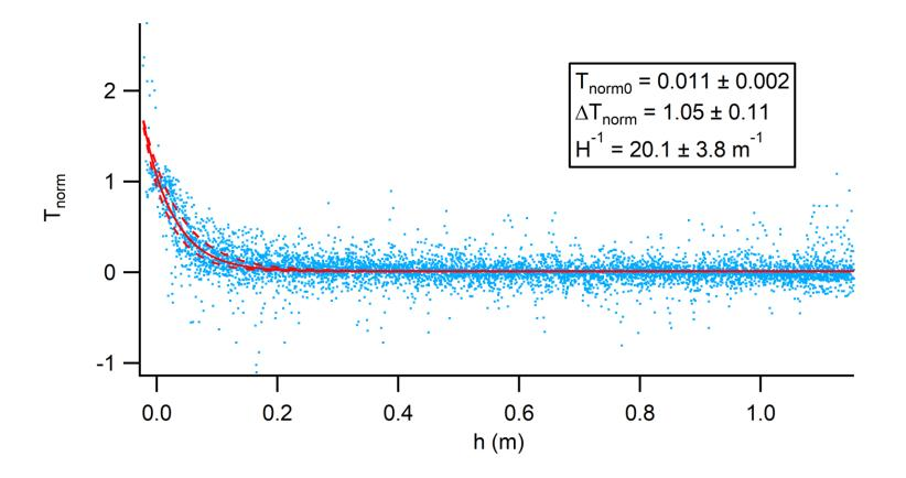
We fitted an exponential function on normalized measurement data (temperature as a function of height) of the form:
