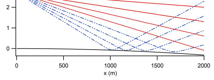
Bending of light rays in air over a water surface with ambient temperature 1°C and water temperature 5°C, on a distance of 2000m. Each ray starts from a height of 2.7m in different angles (-0.16-0.04°) from horizontal in 0.02° steps. The surface of Earth is indicated with a black curve.
