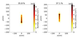
Number density of electrons in the middle of a nanorod of size 25x130 nm at different times. The nanorod is orthogonal to the beam direction, x.
