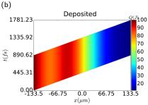
**Deposited energy** per unit time in the space-time plane across the depth, h, of the flat target. (a) without nano-shells (b) with nano-shells To increase central absorption we used the following distribution:
