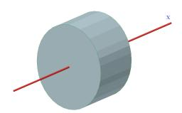
Schematic view of the cylindrical, flat target of radius, R, and thickness, h.  $V=2\pi R^3, \quad R=\sqrt[3]{V/(2\pi)}, \quad h=\sqrt[3]{4V/\pi}.$
