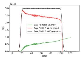
energy in the box **without nanorod** antenna  $3\times10^{-8}$  J (black line) **nanorod** absorbs EM energy reducing it to  $2.3\times10^{-8}$  J (red line) **deposited** energy in the nanorod (green line)
